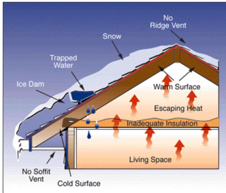
Roof ice dams occur in climates with freezing temperatures and significant snowfall. When the temperature in the attic is above freezing, snow on the roof melts and runs down the sloping roof. When the snowmelt runs down the roof and reaches the colder eaves (overhang) and gutters, it refreezes.
